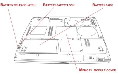
Figure 2-5 The underside of the computer
